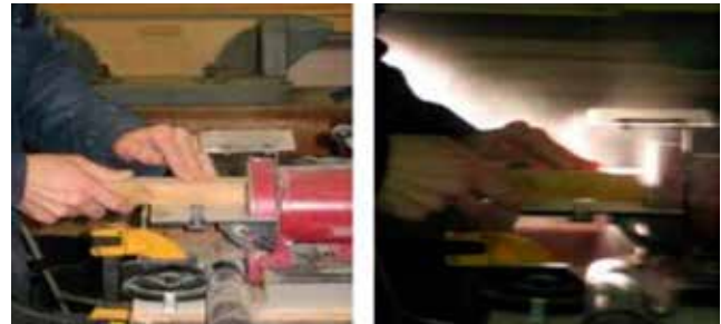
Figure 3 Effectiveness of a dust lamp in showing the dust cloud produced by sanding. This is normally invisible to the naked eye
