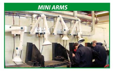
The Mini Extraction Arm is an ideal way of removing a wide range of airborne substances. Weld and solder fumes, dust, vapour and gases are quickly captured at source creating a cleaner and healthier workplace. The Mini Arms may be desk, ceiling or wall mounted.
